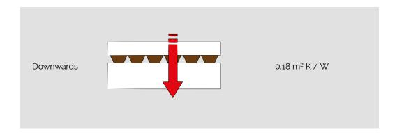
The thermal resistance values are calculated following DIN EN ISO 6946
