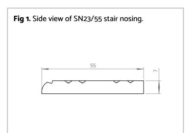
**Item:** AATi™ type SN23/55<sup>®</sup>- HDLT™ anti-slip stair nosing with silicon carbide granules cast into the metal matrix of the wearing surface. This is a protected and registered design:
