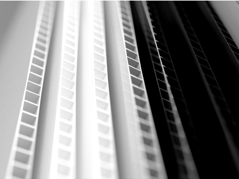
Correx is the original twin wall fluted polypropylene protection board and has become the industry standard for most temporary protection applications, following its launch in 1974. It can be used both internally and externally for a wide range of applications within the construction industry including protection of floors, walls, doors, windows and ceilings and as a formwork material for concrete construction.
