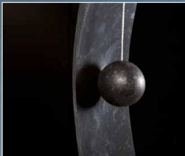
These pictures show that RECYFIX withstands the impact of a hurled steel ball. Here it proves its characteristics of flexibility, toughness and unbreakability.
