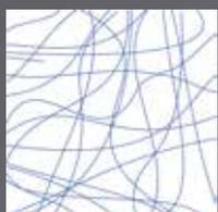
Thermoplast (= basic product for **RECYFIX**): The thermoplasts are made from long molecule chains. They are held together by intermolecular force. This is like joining together, entangling and interlocking. There is therefore no molecular bond between the individual strands. This means that the material can be molten again without molecules having to be destroyed.
