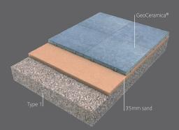
Now GeoCeramica® makes it easy to install porcelain paving over a conventional Type 1 sub-base, for perfect, durable results, every time
