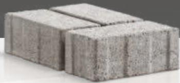
Ecogranite Aquaflow permeable blocks are specially designed, incorporating a slot and chamfer, allowing water to disperse at a high rate. Available in 60mm and 80mm rectangular blocks, they sit effortlessly alongside our conventional Ecogranite Royal Forest paving. The textured surface exposes the sparkling granite offering excellent skid/slip resistance. The Ecogranite Aquaflow permeable block can be specified for all sites designed under BS7533-pt13.
