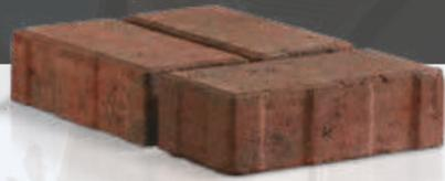
Aquaflow permeable blocks are specially designed, incorporating a slot and chamfer, allowing water to disperse at a high rate helping to prevent localised flooding.
