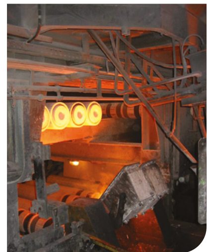
Centrifugal casting process
