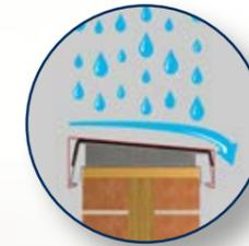
Protects parapet wall and directs water onto the roof area
