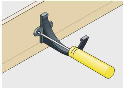
2. Generally, position brackets at 915mm centres allowing additional brackets on either side of where gutter joints will occur.
