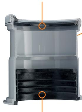
Rubber gasket functions like a bellows to allow for thermal movement.
