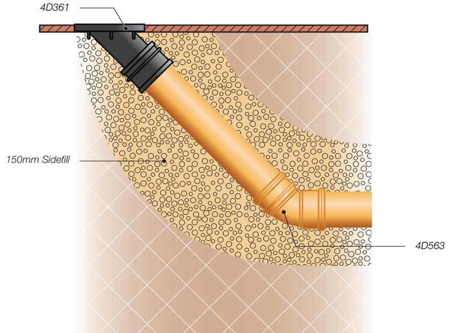
Figure 26: Rodding Eye – intermediate access
