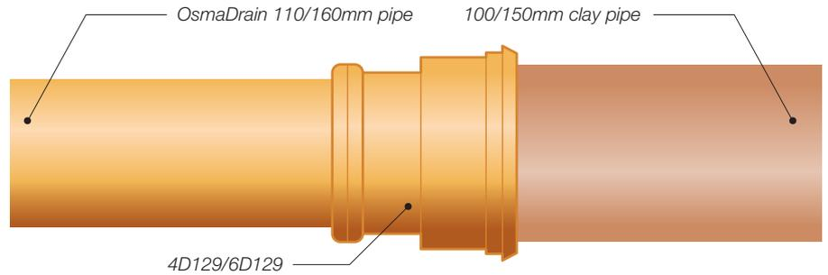
Figure 35: Connection to thick-wall clay spigot
