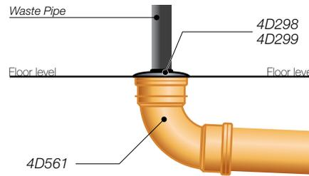
Figure 14: Connection of internal waste pipe at depth
