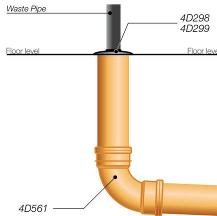
Figure 15: Internal connection of 110mm diameter soil pipe
