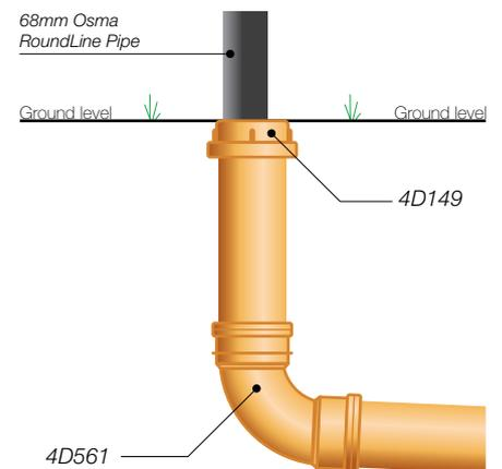
Figure 18: Connection of RoundLine rainwater pipe to OsmaDrain 110mm socket
