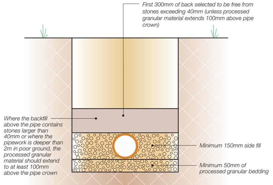
Figure 6: OsmaDrain pipes laid on 100mm minimum of processed granular material
