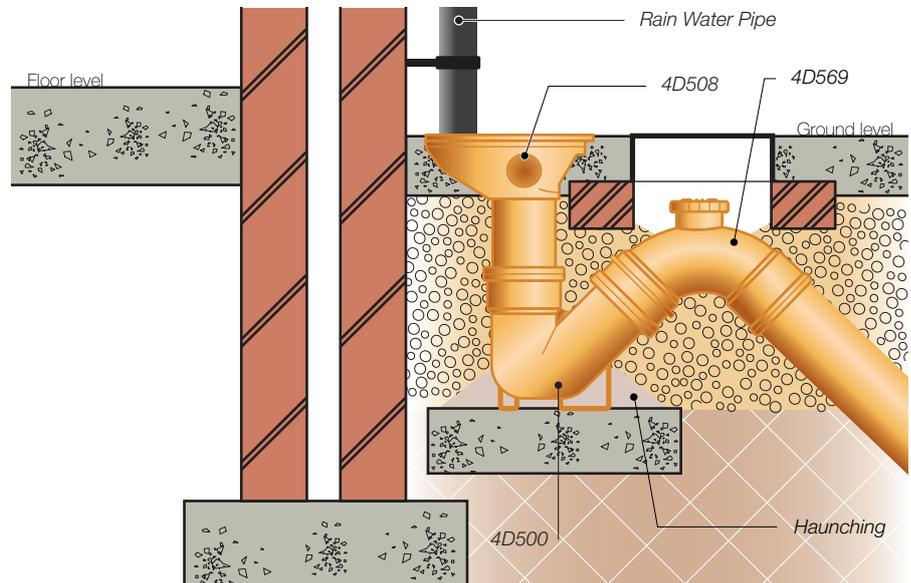
Figure 28: Universal Gully – protection of outlet bend
