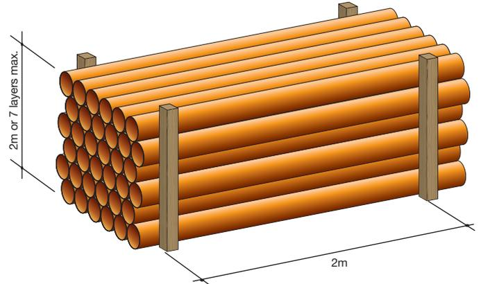
Figure 3: Storage of loose pipes on bearers
