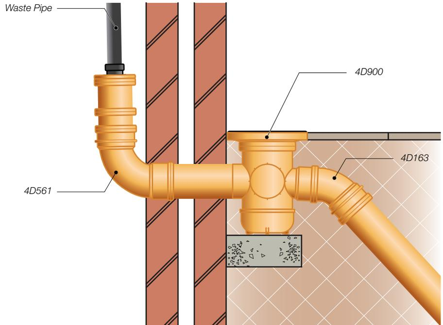
Figure 30: Bottle Gully installation with vertical inlet
