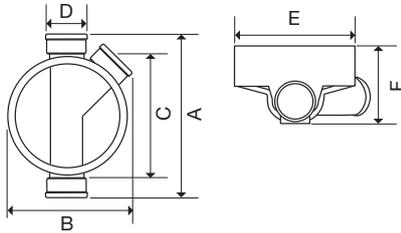
**D/S Equal Shallow Inspection Chamber Base (WAJ 12)**
