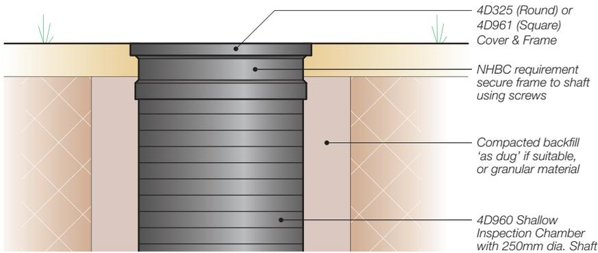
Figure 4: Installation detail Class A15 – For non-trafficked pedestrian applications subject to loading up to 15KN (1.5 tonnes)
