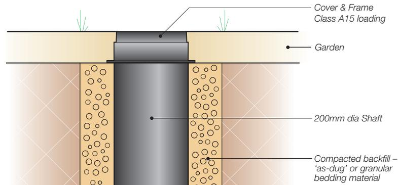
Figure 13: Installation detail A15 – For non-driveway applications subject to infrequent vehicle loading up to 15kN (1.5 tonnes)
