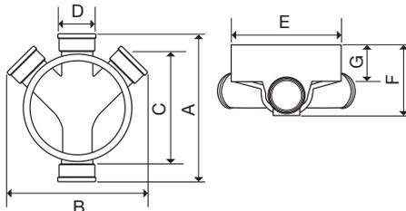
**D/S Equal Shallow Inspection Chamber Base (WAJ 5)**
