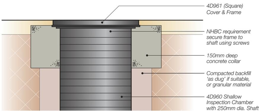
Figure 5: Installation detail – green areas (non-loaded)
