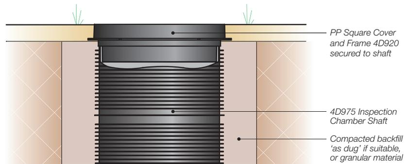
Figure 9: Installation detail Class A15 – areas subject to occasional vehicle loading up to 15kN (up to 5 tonnes when supported with a concrete plinth). For heavier vehicles (ie. Electric vehicles, 4x4s, pick-up trucks & vans), B125 cover should be used
