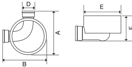
**D/S Equal Shallow Inspection Chamber Base (WAJ 2)**
