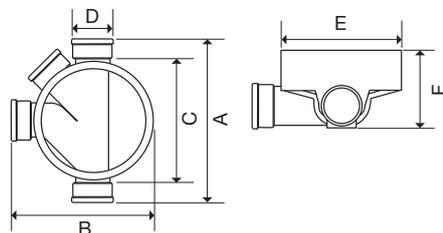
**D/S Equal Shallow Inspection Chamber Base (WAJ 16)**
