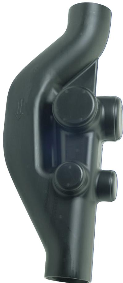
The Wavin HDPE Airmix “Sovent” fitting prevents all this. The principle of this fitting is based on keeping a free path air to leave or to enter the system and thereby keeping the pressure level within acceptable limit.
