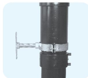
5. Install the pipe and fix with a fixed-point bracket on the socket side and sliding brackets over the rest of the pipe length
