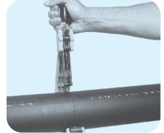
6. Clamp both pipe-ends in the welding machine and ensure correct alignment. Eliminate any bending forces if present.
