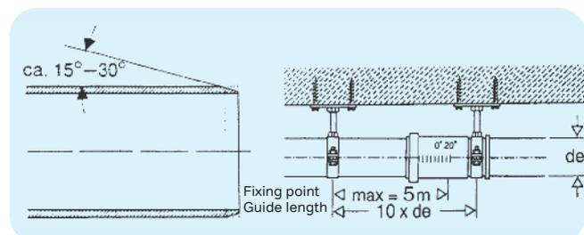
Figure 4: Fixing a long pipe collar
