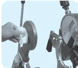
3. Clean the heater plate with HDPE cleaner and a soft cloth. Prevent any damage of the Teflon coating.
