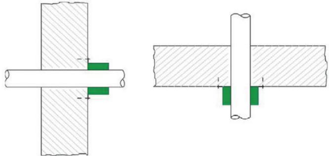
Figure 11: Collar Installation (Both sides of wall)
