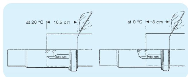
The insertion lengths required are dependent on the temperature of the surroundings during installation. Installation temperatures of 20°C require insertion lengths of 10.5cm; installation temperatures of 0°C require only 8cm insertion lengths.
