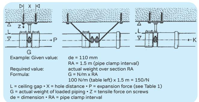
Reduction collars can be used to achieve the required diameters. Fixings used must be capable of withstanding the actual weight of the loaded piping and the resulting tensile forces generated by expansion.
