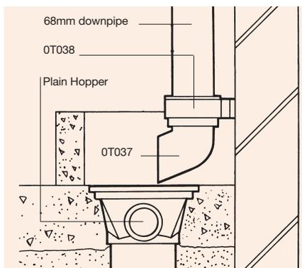
Figure 17: Connection to bottle gully
