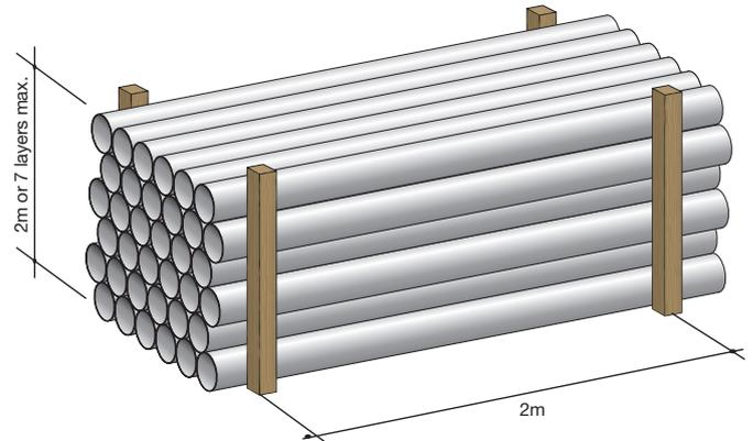
Figure 22: Storage of loose pipe on bearers
