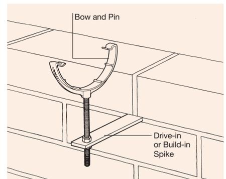
Figure 34: Installation of Rise and Fall Brackets
