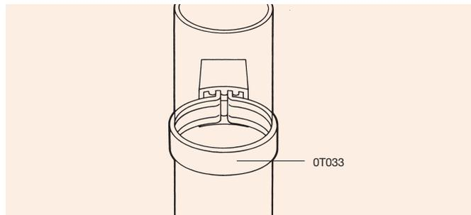
Figure 43: Use of Pipe Bracket Spacer
