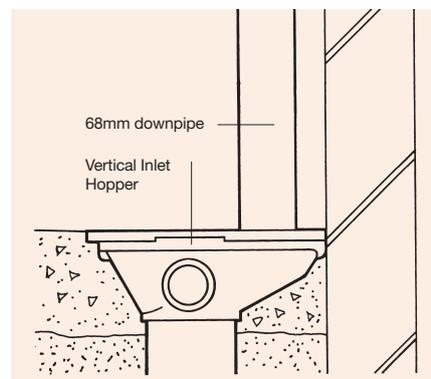
Figure 18: Connection to bottle gully
