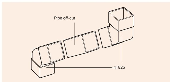
Figure 46: RoofLine shallow offset
