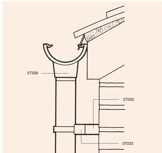
Figure 9: Use of Pipe Bracket Spacer
