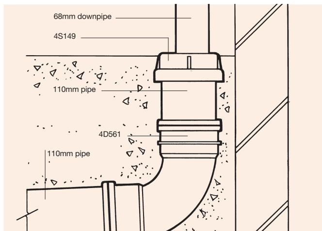
Figure 49: Connection to 110mm PVC-U Socket (61mm square pipe)
