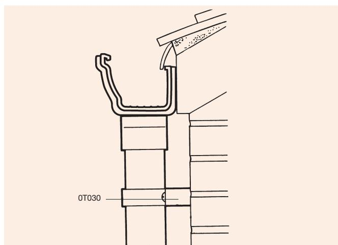
Figure 44: Application of Pipe Bracket Spacer
