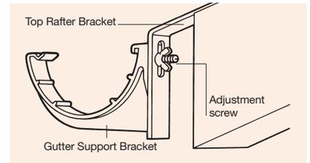
Figure 37: Adjustable Top Rafter Bracket (with SquareLine Union and Support Bracket)
