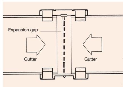
A gutter jointing bracket or gutter union with bracket should be fitted within 300mm from the end of terminal lengths of gutter.
