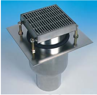
Gully 5150 Vertical Outlet Flow Rate 1.8 l/s Outlet diam. 85, 110mm
