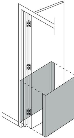
Large size formed angles for protection of door edges and faces.
