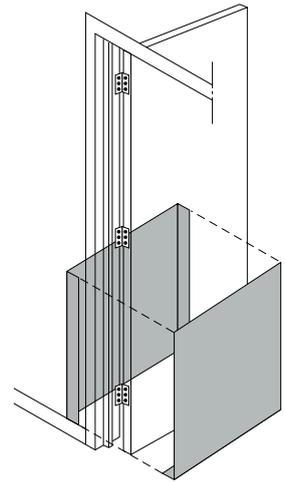
A solution for humid or wet environments consists of an angle and a channel to cover door faces and edges, including the bottom door edge.
