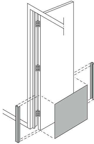
A combination of channels and plates for protection of door edges and face(s).
