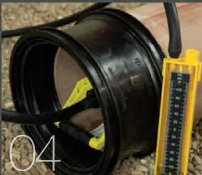
04 Apply pressure to achieve a 110mm water gauge on the manometer
