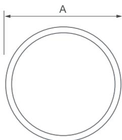
**Chamber Base to Shaft Seal**
