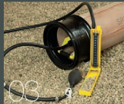
03 Connect a "U tube" gauge (manometer) to the testing stopper
