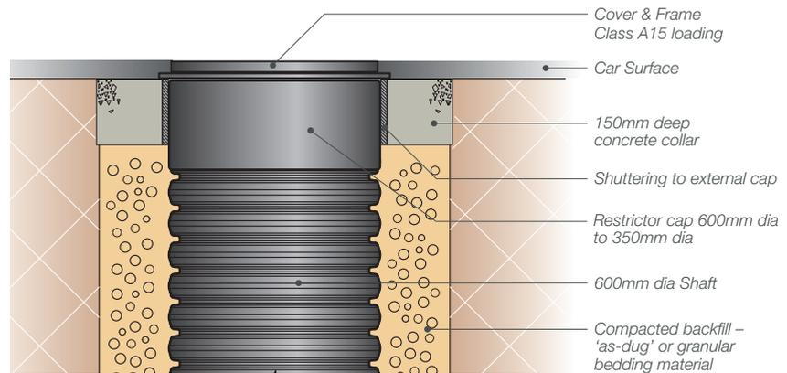
Fig. 36 – Installation detail B125 loading – paved areas with limited traffic load
