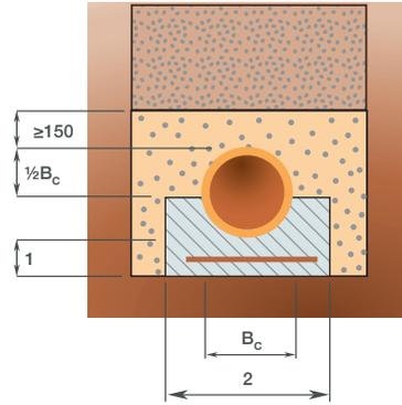
b. Reinforced concrete bed. Bedding factor 3.4 (0.4% steel)
