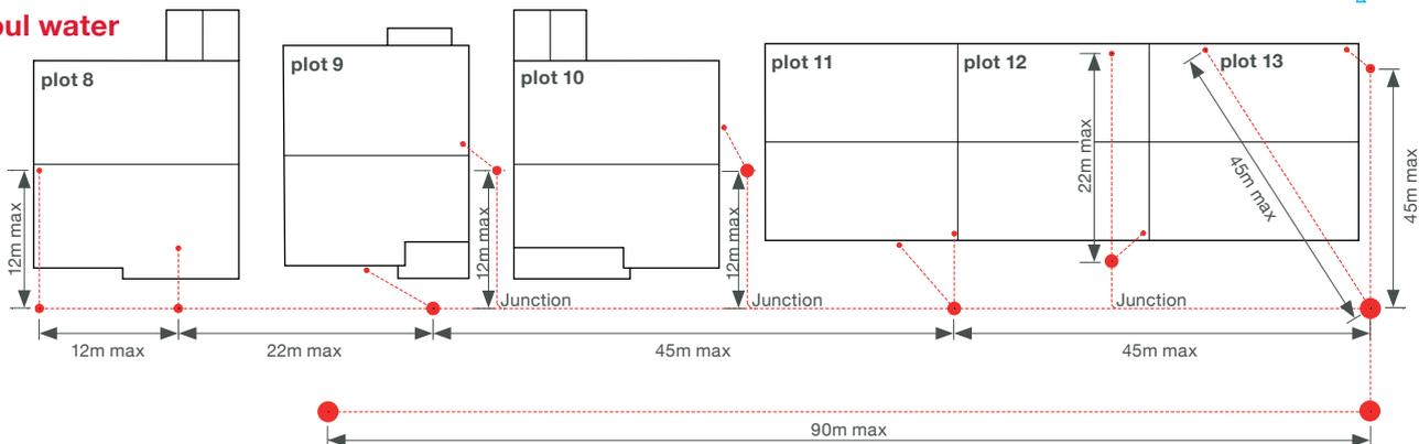
This drawing is to illustrate the recommended maximum spacing of access provision (in metres) for manual cleaning only. Diagrammatic only – not to scale.
