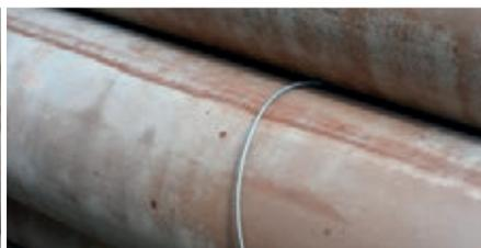
Do NOT cut the metal wires at any time on SuperSleve pipe packs.
