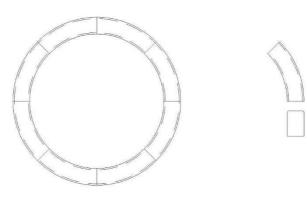
**Dimensions** Internal diameter 2400mm, External Diameter 3000mm
