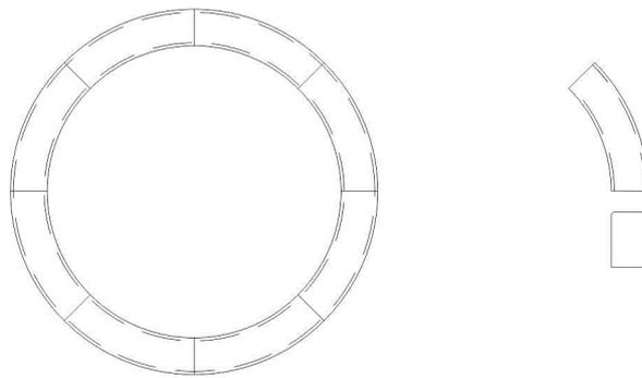
**Dimensions** Internal diameter 2400mm, External Diameter 3000mm
