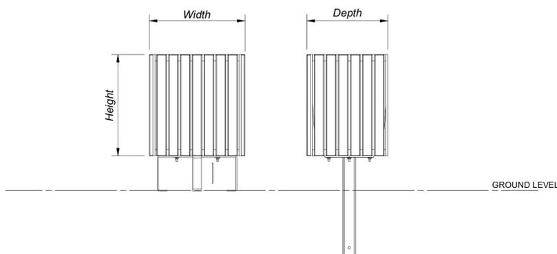
**Dimensions** Width - 390mm, depth - 340mm, height - 476mm excluding fixings (sizes are approximate)
