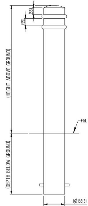
A substantial bollard with a clean appearance, the GFC6R Ornamental Bollard is constructed from mild steel and galvanised to ensure its longevity. Caps and rings of cast iron are welded on to the steel body to complete the design.
