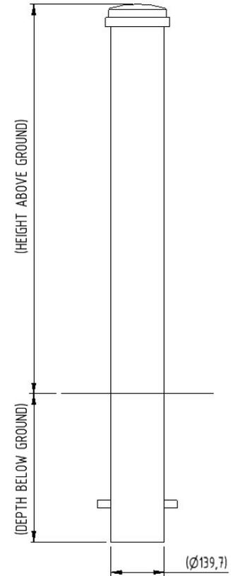
A substantial bollard, with a simple, clean appearance. The GFC9000 Ornamental Bollard is constructed using mild steel, galvanised to ensure its longevity. A decorative welded steel cap is added to complete the design.
