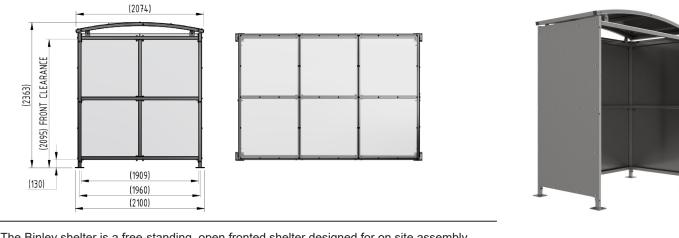
The Binley shelter is a free-standing, open fronted shelter designed for on site assembly, constructed from galvanised mild steel. Complete with galvanised sheet roof, and side panels. Side-to side curved roof.
