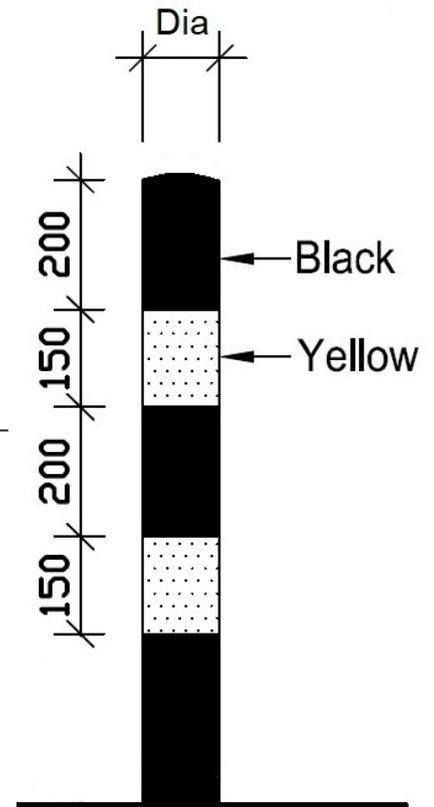
The AUTOPA range of Black & Yellow bollards are ideal for providing high visibility protection in both internal and external warehousing environments. All products in the range are galvanised mild steel, ensuring their longevity and are designed to take the knocks and bumps that occur in all warehouse environments.
