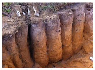
TamCrete UFC range of ultrafine cements incorporate selected granulated blast furnace slag and Portland Cement as an activator. TamCrete UFC cements are ideally suited for permeation grouting into soils due to their fine particle size or injection into tight rock formations.
