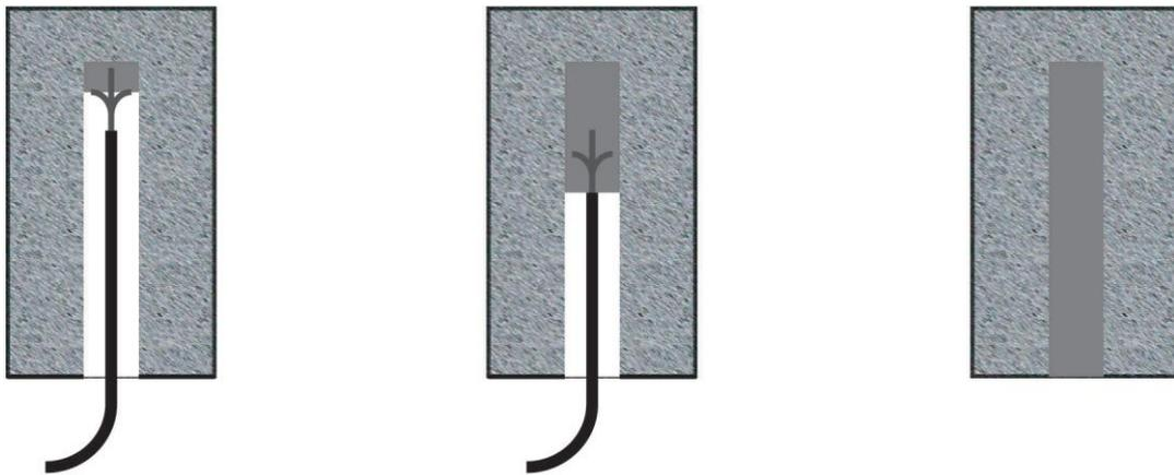
1. Pump the cement grout with hose from bottom until the hole is completely filled.
