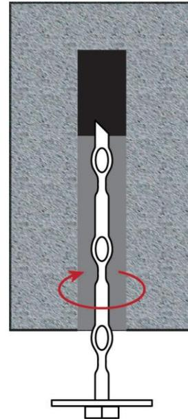
3. Continue to spin the bolt for at least 5-10 revolutions after the bolt reaches the bottom.
