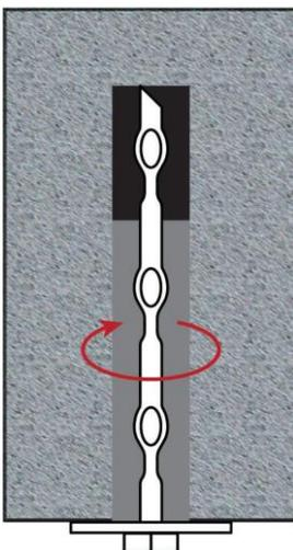
4. Stop rotation and hold the bolt until the FAST resin hardens and then rotate the nut to apply a small tension load.
