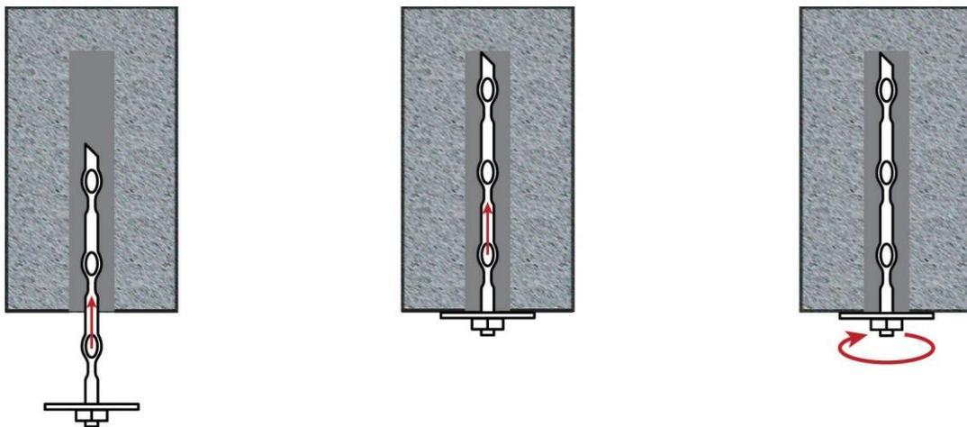
2. Insert D-Bolt® up to the bottom of the borehole according to the installation procedure.
